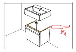
Having finished all plumbing connections, secure the basin to the unit using a silicone sealant. Make sure the basin is correctly aligned with the furniture and allow the sealant to dry. The silicone sealant will help the basin sit level on the furniture and protect the unit from water damage.
