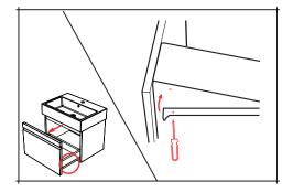
To remove the drawer from the unit, fully extend the drawer. On the underneath of either side of the drawer are two screws that can be undone to release the drawer from the runners. The drawer can be returned in the same way.
