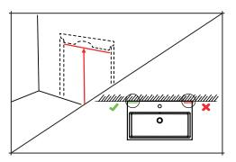
Mark the location of both mounting plates ensured that they are positioned inside the sidewalls of the unit. The recommended height for the unit including basin is 900mm.
